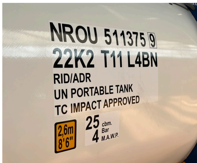
Dual specification markings (RID/ADR L4BN – UN Portable T11)
